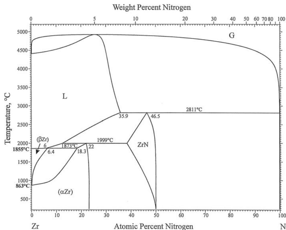
**Fig. 1** N-Zr phase diagram
